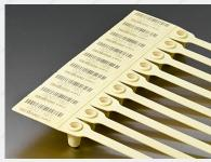
A Fix Length Security Seal with a unique designed locking jaw to seal Tote boxes, Truck doors, Trailers and Containers. Used in industries such as Logistics, Railway, Retail and Transport. Easy to control due to its special breaking point which is clearly visible outside of the housing. Easy to close and break. Closed chamber to encapsulate locking tip upon removal to restrict reuse and tampering of seal.
